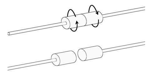
6. Place the fuse inside, then twist the two sides of the holder to the right to bring it together and secure the fuse in place.
