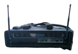
6. Switch on the Radio Frequency Transmitter and 2 Channel wireless microphone receiver. Ensure that all necessary switches are ON.
