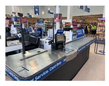
hybrid checkouts in their stores, which are a combination of both a self-service and a manned checkout. The display screen in the middle can be rotated 180 degrees so it can be used in a self-service position or turned so that a member of staff can man the checkout, assisting shoppers in scanning and paying for their items.
